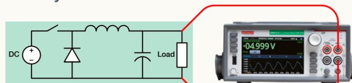
Power-up/power-down test connections.
