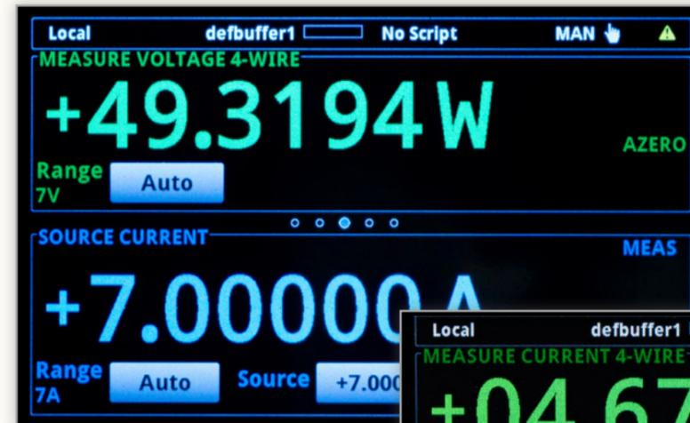
Instruments like the 2450 SourceMeter SMU Instrument can display power and solar cell max power, short circuit current, and open circuit voltage.
