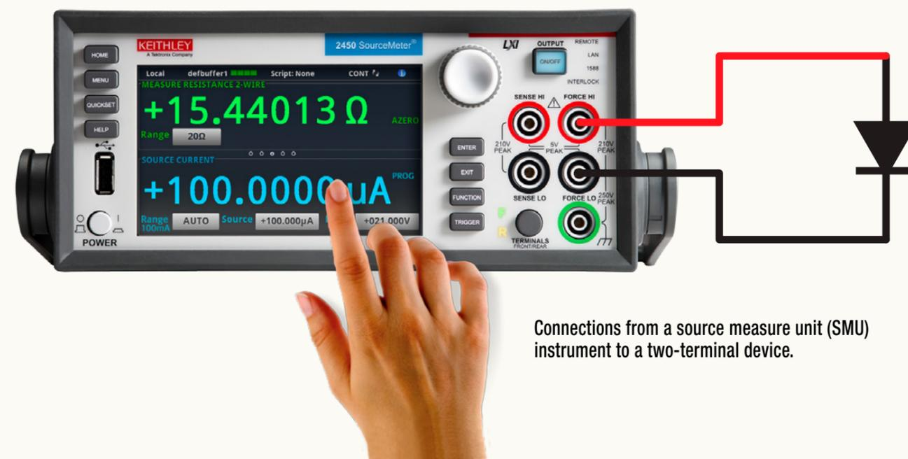
Connections from a source measure unit (SMU) instrument to a two-terminal device.
