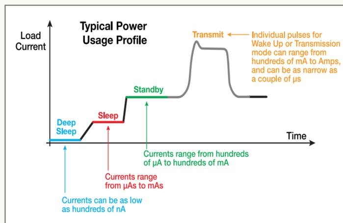
is a non-trivial task, since these devices often draw current in wide ranges from nano-amps to amps depending on operating modes and often have short wake up times, as well, that can last for as little as a few microseconds and require extensive data logging periods to capture a complete power usage profile.
