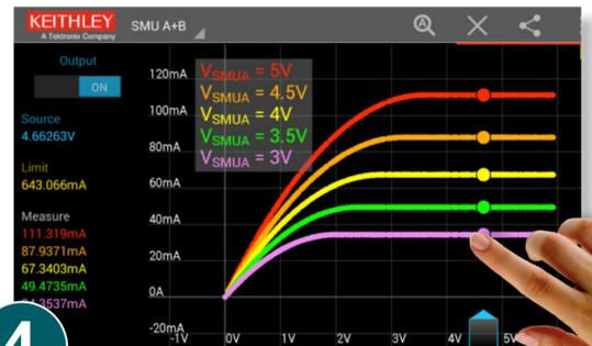
Tablet-based applications, such as Keithley IVy, provide immediate visualization and control of a three-terminal "family of curves."
