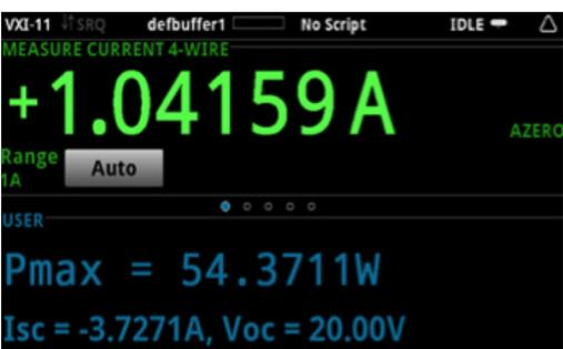
**5** Some instruments can directly display power and solar cell max power, short circuit current, and open circuit voltage.
