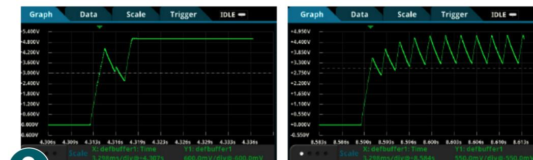
**6** Examples of power-up anomalies (temporary output voltage dip on the left and permanent failure to power-up on the right.)
