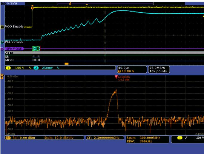
Figure 2 - Spectrum Time is moved about 60  $\mu$ s to the right. At this point, the spectrum shows that the PLL is in the process of tuning to the correct frequency (2.400 GHz). It has made it up to 2.3168 GHz.
