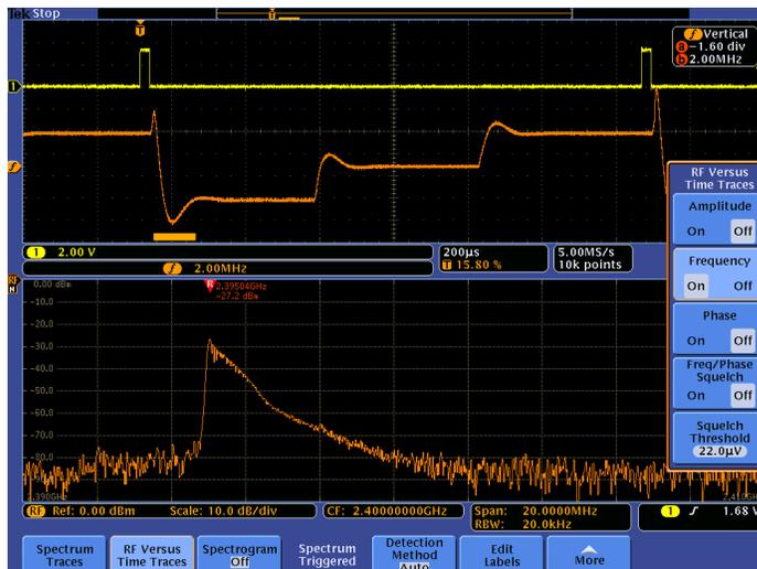
The orange waveform in the Time Domain view is the frequency vs. time trace derived from the RF input signal. Notice that Spectrum Time is positioned during a transition from the highest frequency to the lowest frequency, so the energy is spread across a number of frequencies. With the frequency vs. time trace, you can easily see the different frequency hops, simplifying characterization of how the device switches between frequencies.
